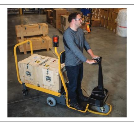
If you're working towards reducing your fleet size, towing carts like Dex Pro+ work best for intra-facility material transport. Motorized towing and tugger carts provide safer alternatives for workstation areas. They're smaller and can pass through traffic and aisles with better control than forklifts. Containing forklifts when possible and using carts to deliver materials increases warehouse efficiency and promotes safety.
